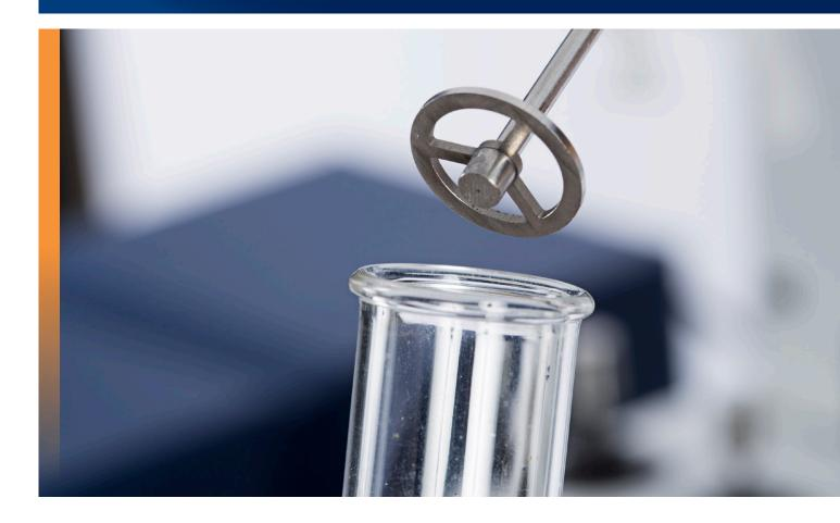
Alphatec™ FNº gives grain receivers a safer and modern way of performing the standard Falling Number test that is used to check sprouting damage in grain and enzyme-activity in flour prior to baking, malting etc.
